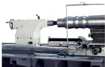
Copy device with 120mm stroke length
